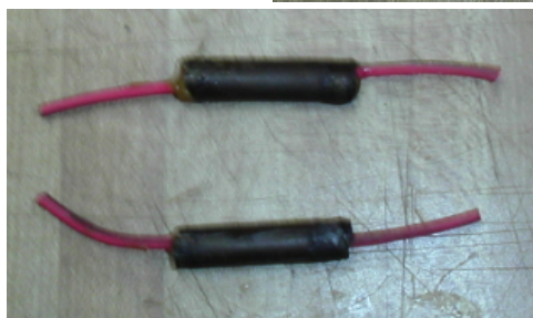
Paper Capacitor Re-stuffing
