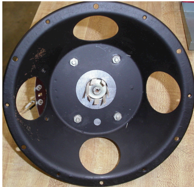
Speaker Electromagnet Centered In Housing
