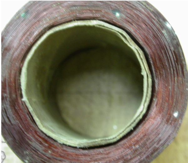
Field Coil With Corroded Windings
