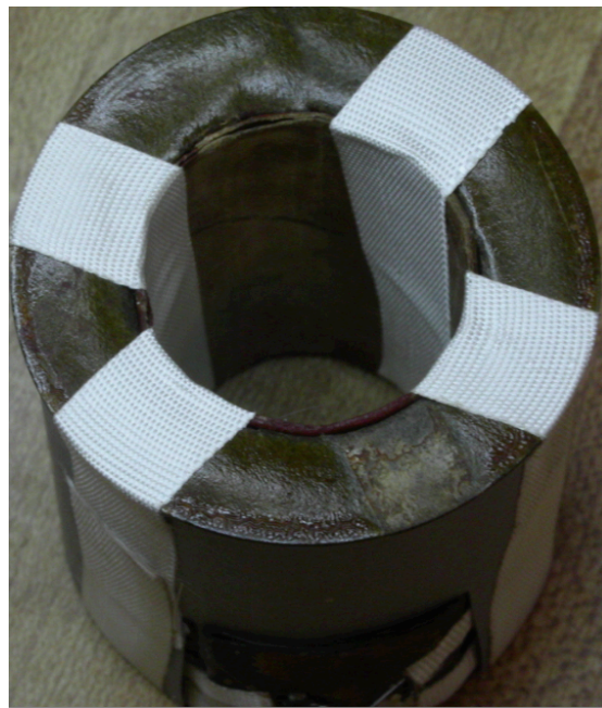
Restored Field Coil
