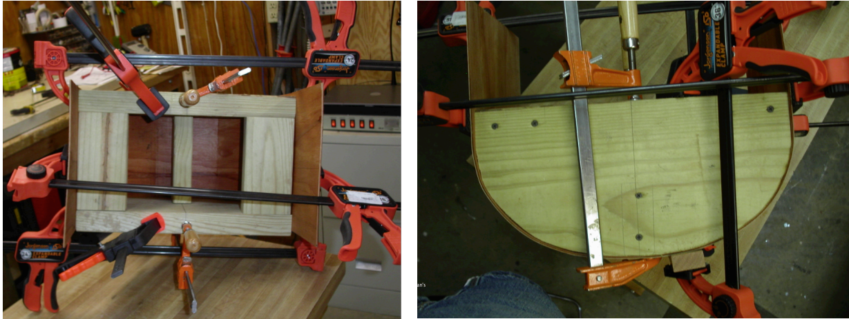
Forming Cabinet Shell
