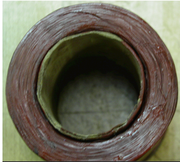
Repaired Field Coil Wires
