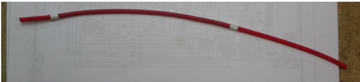
Rubber Core After Winding with Nichrome wire
