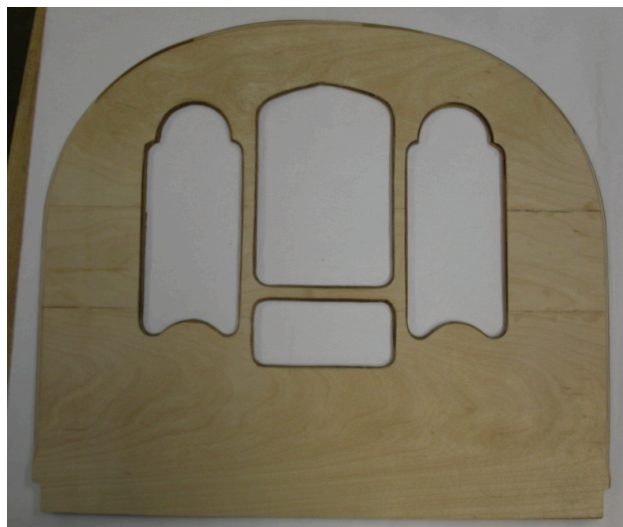
New Front Core Showing Added Birch Veneer
