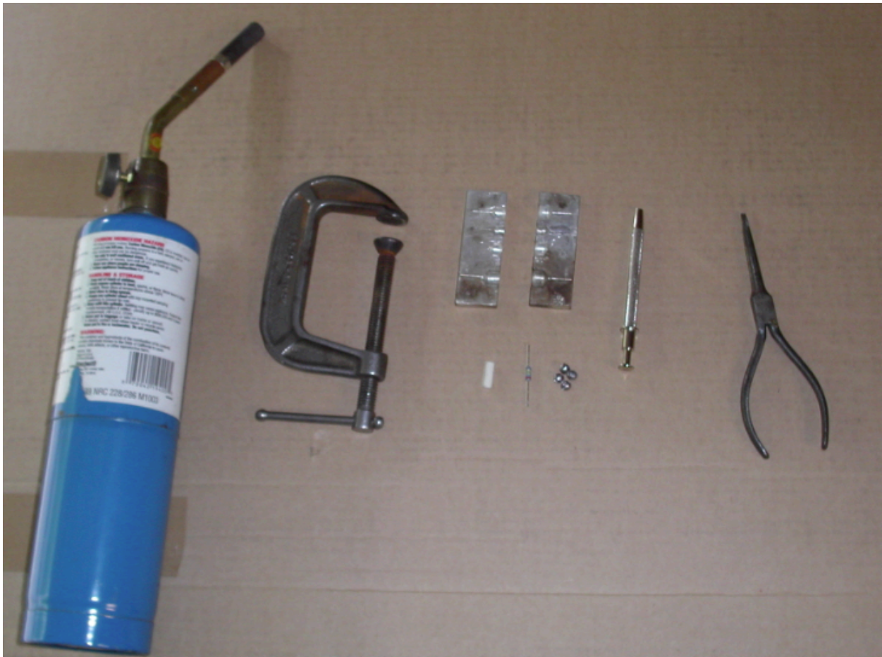
Materials Used To Make Reproduction AK Ceramic Resistors
