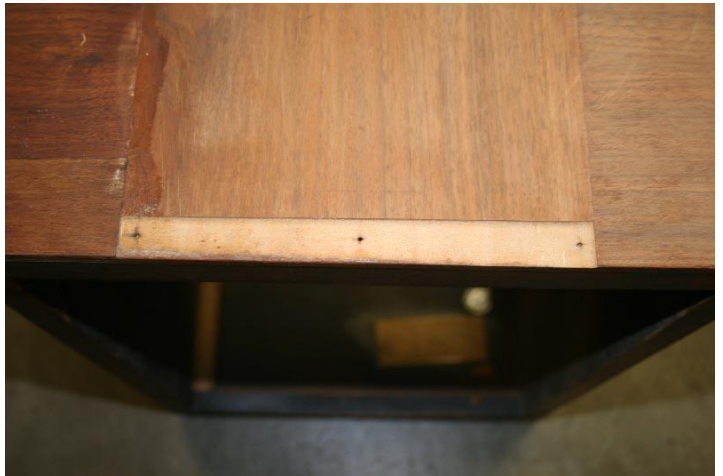
Damaged Veneer Removed
