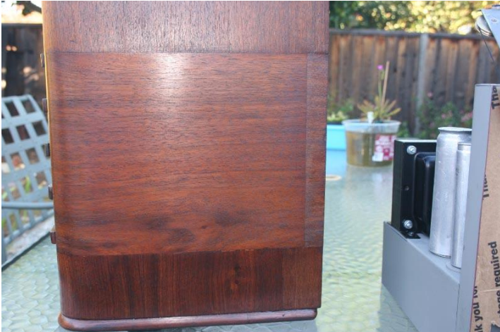
Veneer Replaced & Finished
