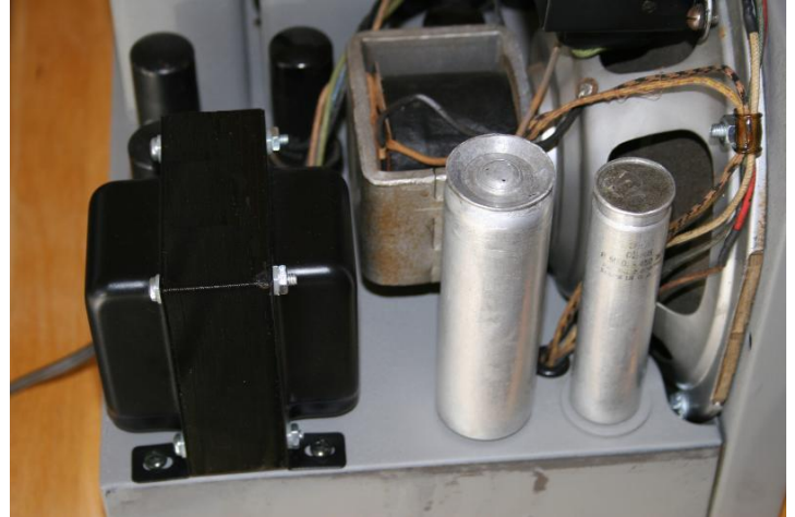
Installed PWR Transformer
