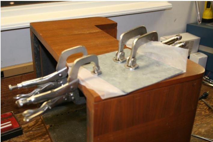
Cabinet Top Veneer Repair
