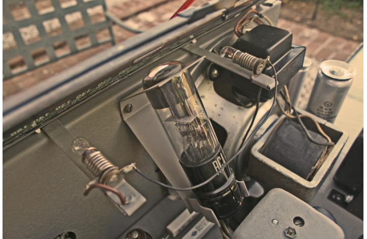
Pilot lamps restored
