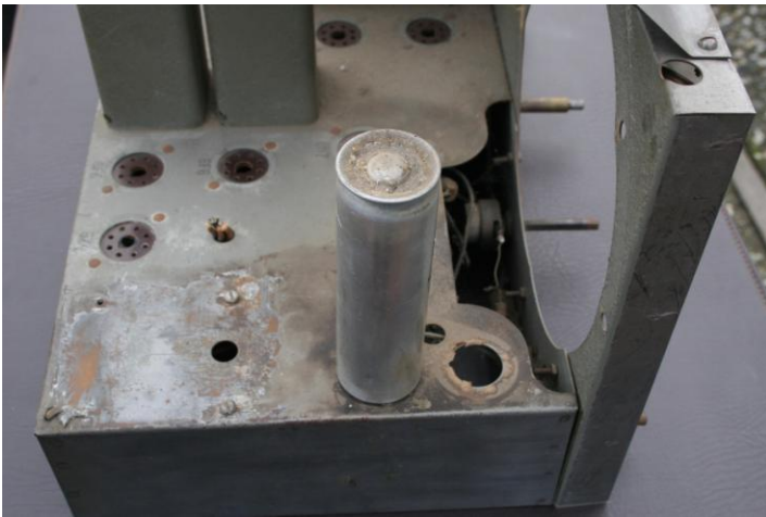
One Missing & One Very Bad Capacitor
