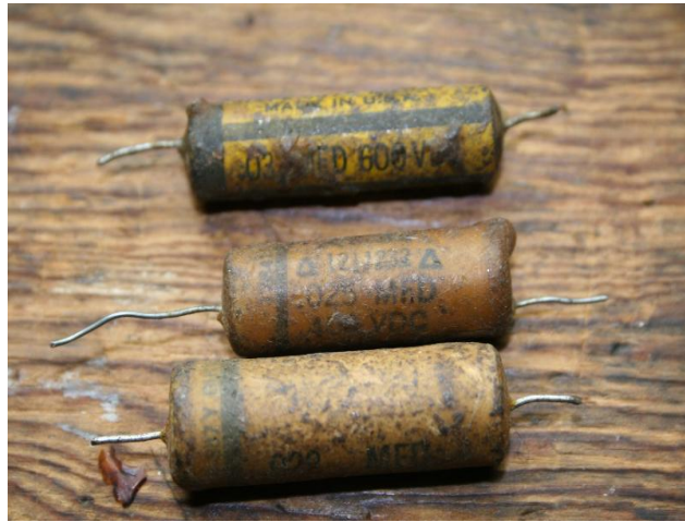
Replacement Capacitors before re-waxing
