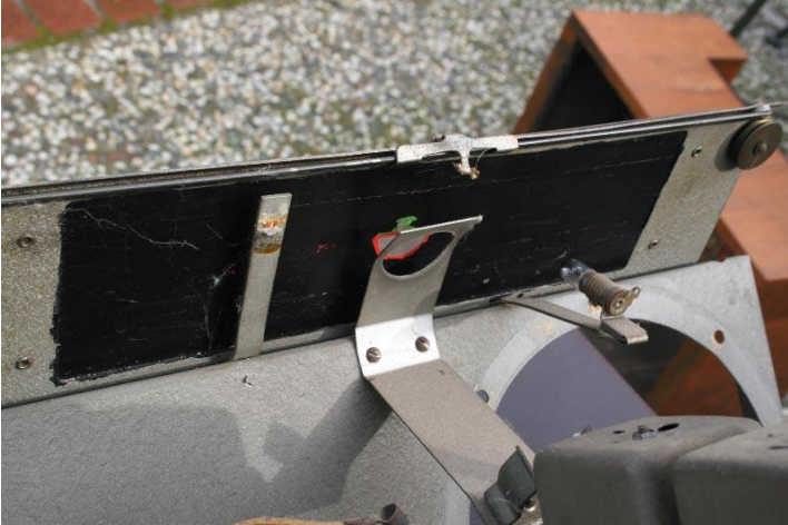
Pilot lamp missing bracket bent
