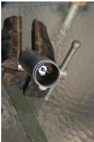
New Capacitor Installed in Can
