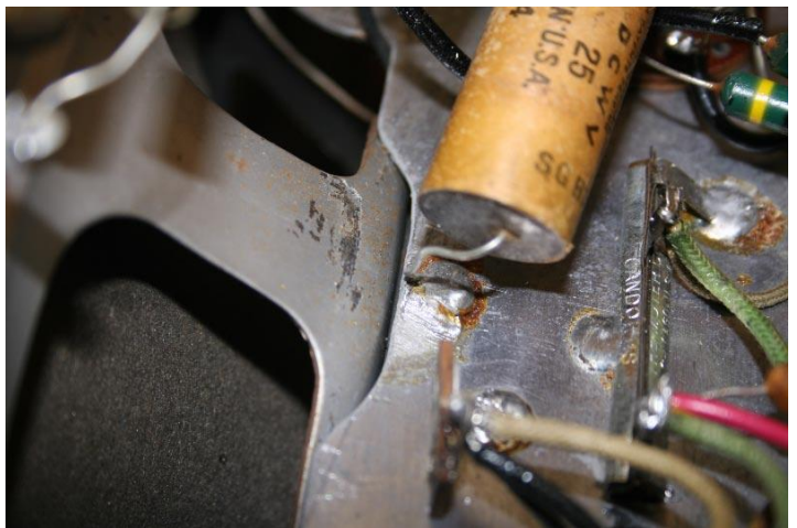
Chassis relieved to Accommodate New Speaker
