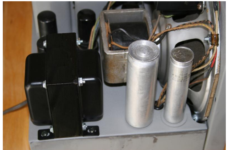
Both Rebuilt Caps Installed
