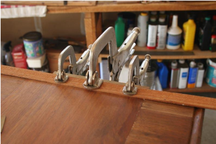
Replacement Veneer Glued
