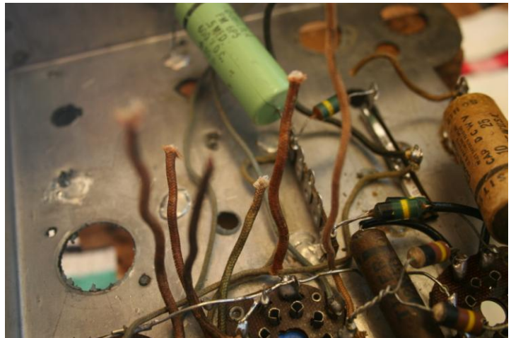
Cut Wires Under Chassis
