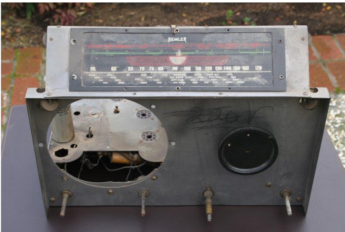
Dial Cord Missing & Broken Cursor
