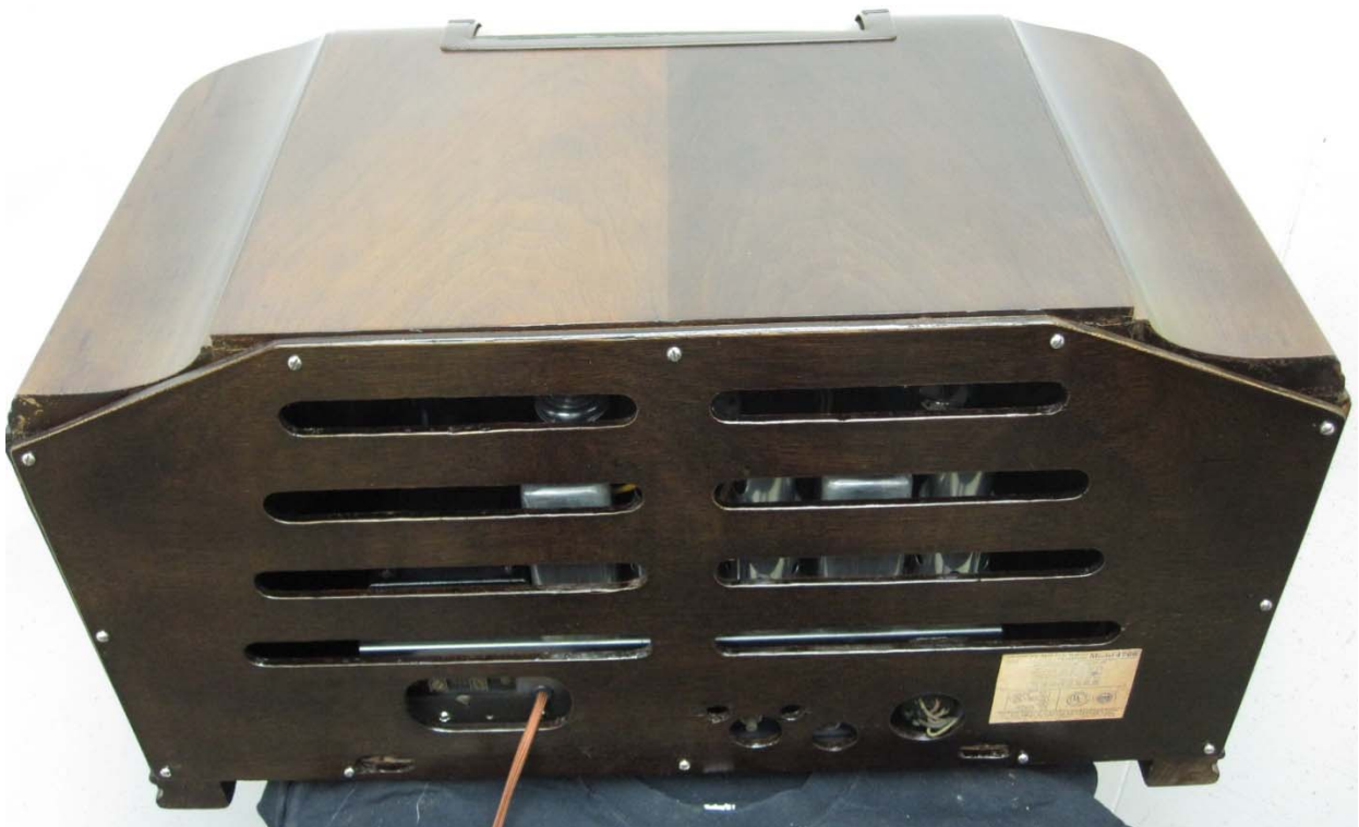
Above: Reproduction rear panel (prototype from the SPARC museum top, reproduction panel below). Below: reproduction panel fitted to the set
