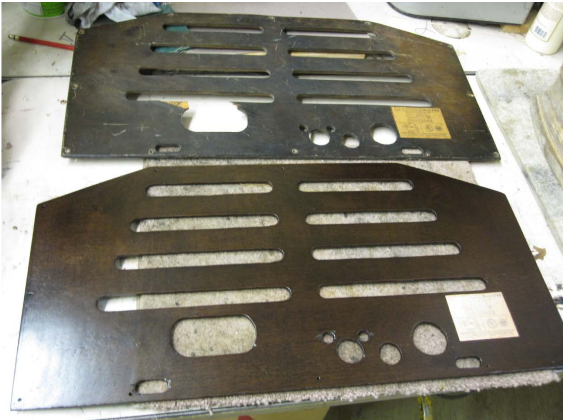
Above: Reproduction rear panel (prototype from the SPARC museum top, reproduction panel below). Below: reproduction panel fitted to the set
