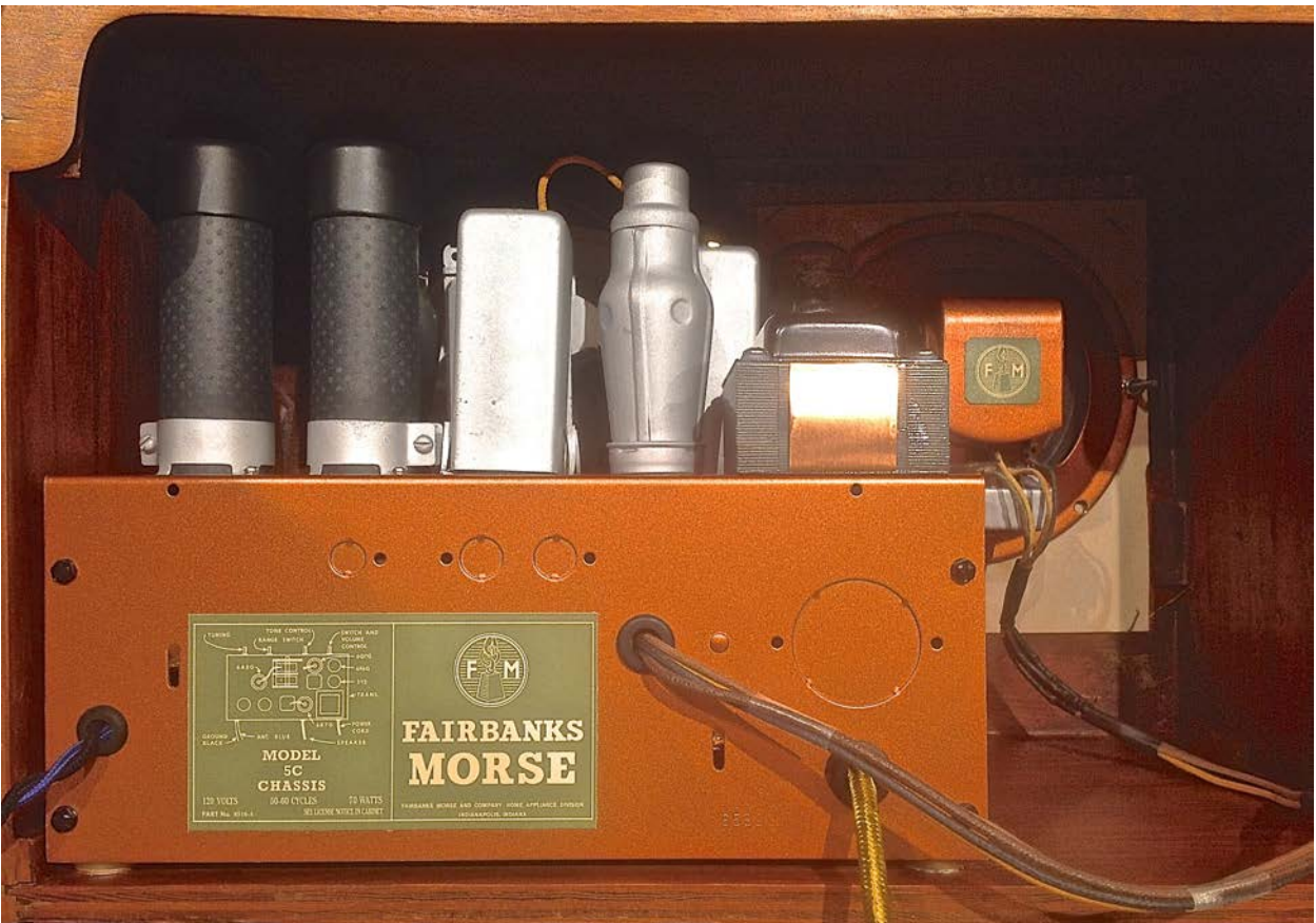
Cabinet complete, speaker is mounted and connected to the chassis circuit. Chassis is mounted with new grommets and bolted to the cabinet using original screw bolts. Decal has been replaced.
