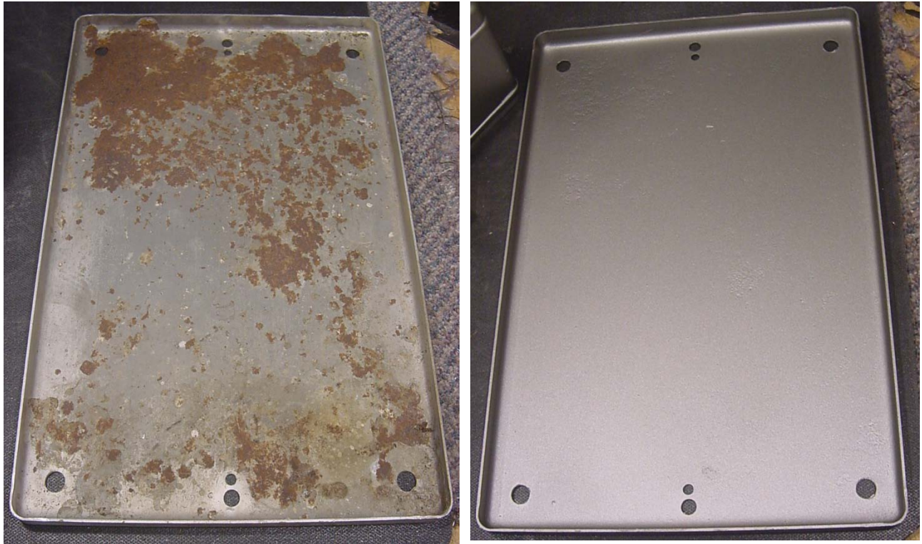
Above: chassis bottom plate as-found/restored, Below: chassis rear plate as-found/restored
