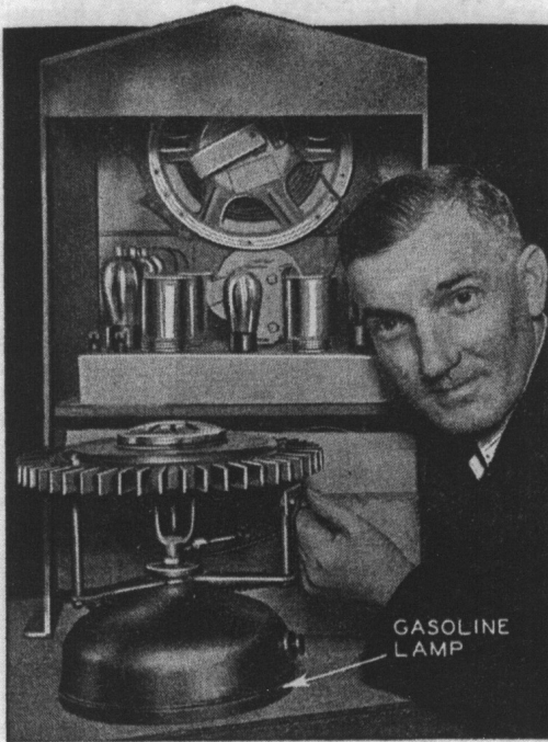
With this new device secret metal alloy is heated at points of contact with kerosene or gasoline to generate sufficient voltage to operate 2-volt tube radio receiver.
