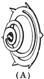
FIG. 27-60.—(A) commercial phosphor-bronze helical coil spring for "grounding" the hub of the front wheel to the front "axle" in order to eliminate front tire "static".
