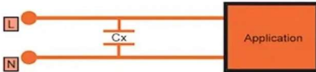
Class X Capacitor (Line - to -Line)
